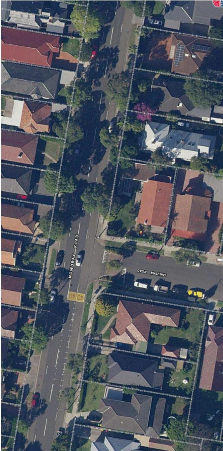
Example – 2 Integrated pedestrian crossing / speed calming measure Corner of Chiltern Road and Mowbray Road Willoughby
