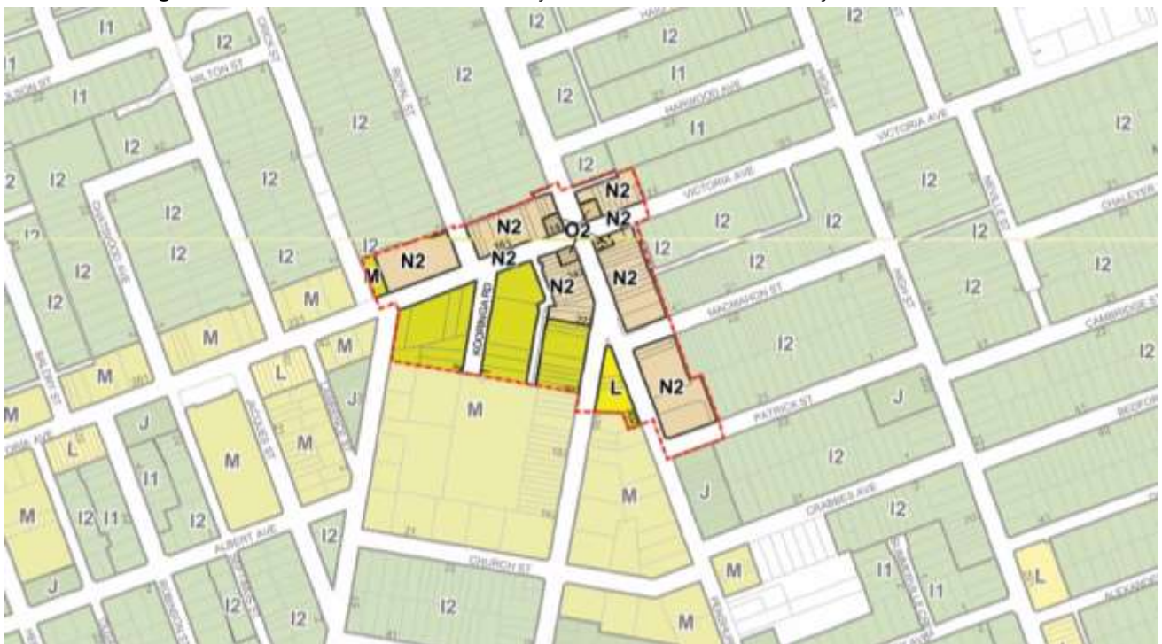
Current height of buildings: Most of the centre is subject to a maximum height of 14m (N2). Buildings at the intersection of Victoria Ave and Penshurst St are allowed a maximum height of 15.5m (O2) while the convergence of Penshurst St and Sydney St is subject to a height of 11m (L). R3 zoned land allows a height of 12m (M).
