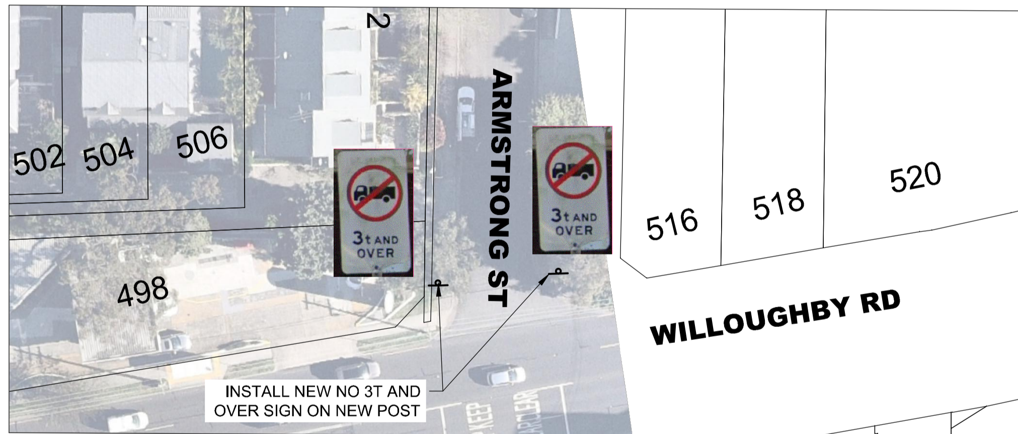
PLAN - NO 3T AND OVER SIGNAGE INSTALLATION ARMSTRONG ST AND WILLOUGHBY RD SCALE 1:400
